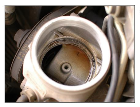
With the filter out, you can remove the remainder of the fluid in the reservoir.
