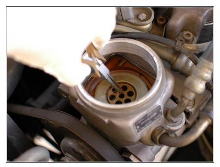
• Remove the filter using a pair of needle nose pliers.
