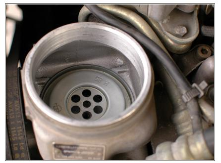
• Install your new filter. Install it with the holes facing upwards, as shown.
