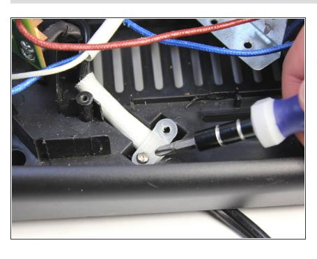
Upon removing the chassis, look in the toaster base to find the little white tab holding the power cord in place. Use a Philips screwdriver to remove the two 10mm screws.
