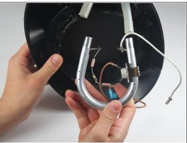
Separate the tubing from the heating coil by grasping the tubing in one hand and the heating coil in the other and gently pulling apart.
