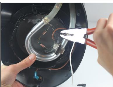
Use pliers to pinch and loosen the crimps.
