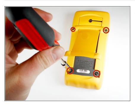
Use your Phillips #2 Screwdriver to remove the four black 21 mm Phillips #2 screws.
