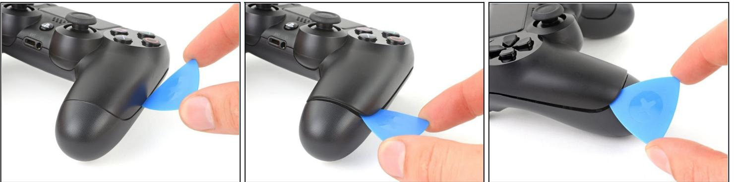
ⓘ Six plastic clips secure the rear case to the front case. The next four steps demonstrate how to release these clips before you can open the controller.
