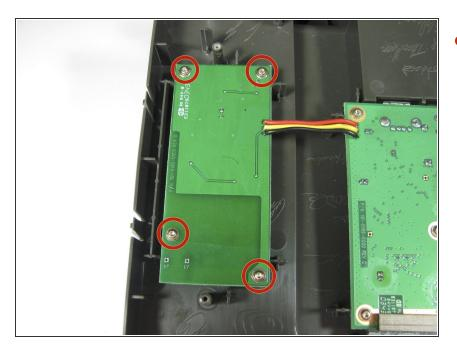
Remove the four 7mm Torx T6 screws.
