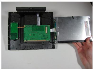
Lift up the display from the left edge and flip display over.
