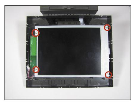
Remove the four 7mm Torx T6 screws.
