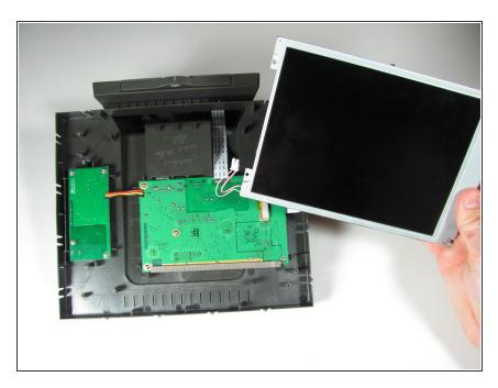
Remove the display assembly from the device.
