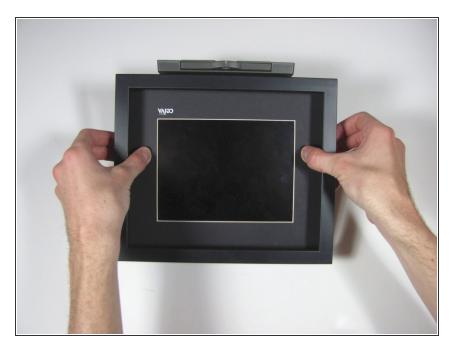
Lift up the frame with your fingers and push down the rest of the device with your thumbs.
