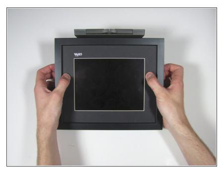
Grip the frame with your fingers under the edge of the frame, and thumbs pushing down on the front of the device.
