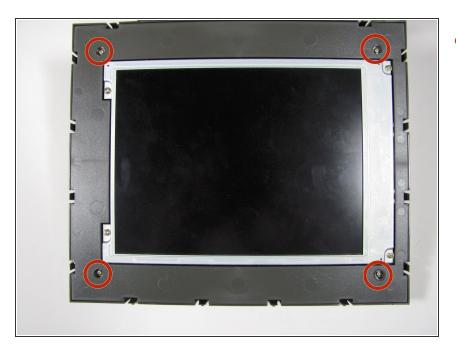
Remove the four 7mm Torx T6 screws.
