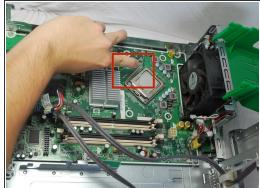
Using your finger, push the lever, located on the right side of the CPU, down and out.
