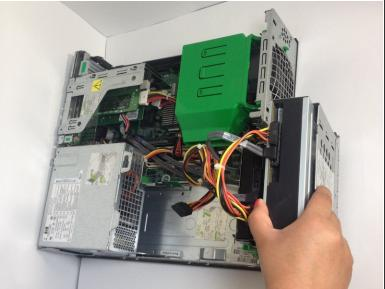
• Using your right hand, grip the CD drive and lift it up to a 90 degree position.
