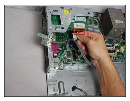
Use your right hand to remove the cable that is attached to the COMS card by grasping the cables and pulling it out.
