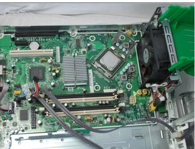
Using your index finger, lift up the bracket surrounding the CPU.
