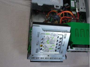
Using your hand, grip the Optical Drive and lift it up into a 45 degree angle.
