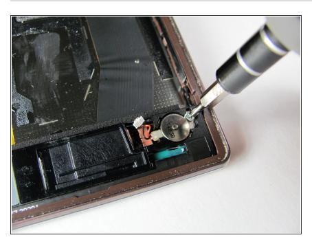
Remove the single 3 mm screw, set next to the vibrate motor, using a Philips #000 screw driver.
