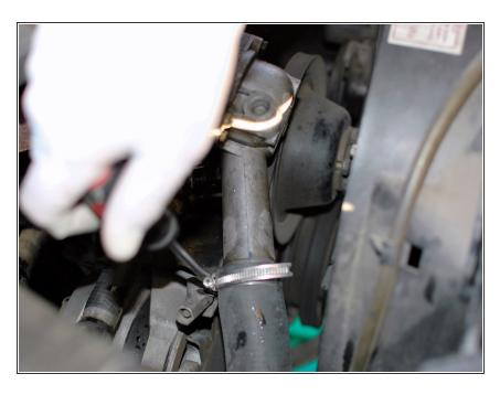
Continue by loosening the clamp on the lower radiator hose where it connects to the thermostat housing.
