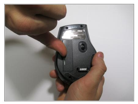
Remove the battery cover with a plastic opening tool, nylon spudger, or a fingernail.
