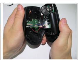
Pry the panels apart gently using a plastic opening tool or spudger.
