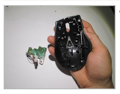
Remove the board from the housing unit and place it aside.
