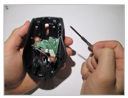
Remove the two screws holding the board in place using a Phillips #0 screwdriver.
