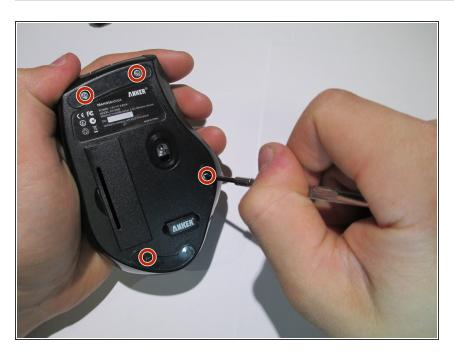
Using the Phillips #0 screwdriver, remove the four screws from the bottom of the mouse.
