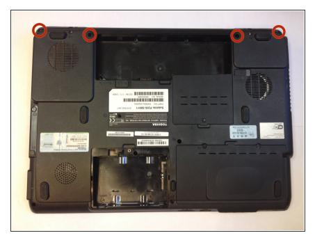
Remove the four 8mm Phillips #1 screws located on the corners below the monitor.
