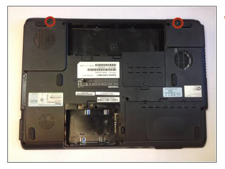
Remove the two 4mm Phillips #1 screws located between the screws removed in the last step.
