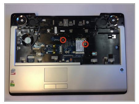
Remove the 2 silver 6mm Phillips #1 screws from the middle of where the keyboard was removed
