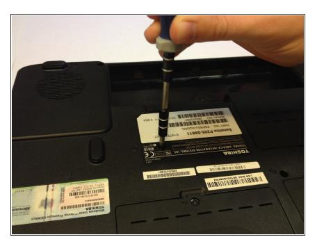
Remove the 8mm Phillips #1 screw that holds the disk drive in place.
