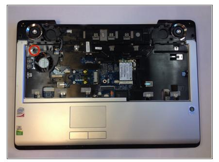
Remove the black 20mm Phillips #1 screw from the top left of the keyboard area.
