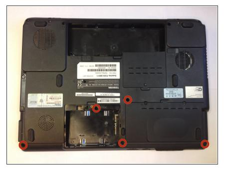
Remove the five 8mm Phillips #1 screws from the bottom of the laptop.
