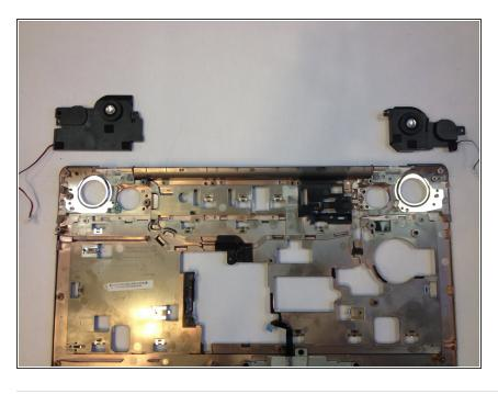
Lift and remove the speakers from the top panel.
