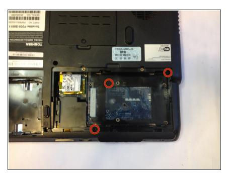
Remove the three 8mm Phillips #1 screws from the bottom right compartment.
