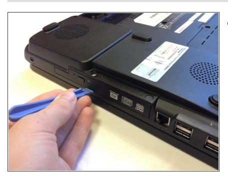
Use a plastic opening tool to pry out the disk drive.
