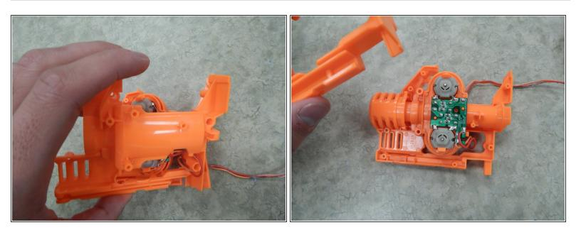
Remove the top shell of the motor casing. This should reveal the inner workings of the motor.
