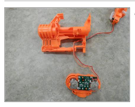
Remove the wiring from the motor by disconnecting the wires from the circuit board.
