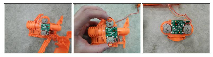
With the shell now removed, locate the motor and controlling circuit board. With your index finger and thumb, squeeze the holders shown in Figure 2 and pull upwards to release the motor module from the rest of the motor's casing. Your motor should be detached from the casing, as shown in Figure 3.
