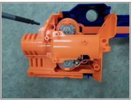
• With your gun disassembled, locate the motor around the front portion of your gun as shown in Figure 1. Remove the two 9.0 mm Phillips screws securing the top shell of the motor casing.
