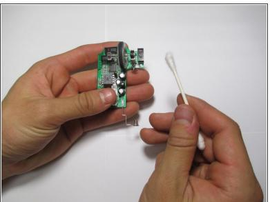
Take a cotton swab and lightly remove any dirt or debris around the pin connections of the scroll wheel.
