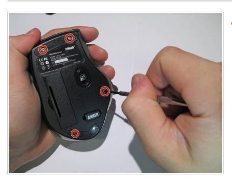
Remove four screws using a Phillips #0 screwdriver.
