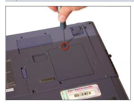
• Remove the screw holding the RAM cover down.
