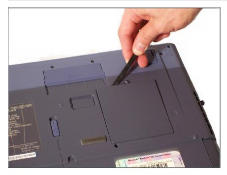
• Use a spudger to lift the covering, revealing the RAM modules inside the computer.
