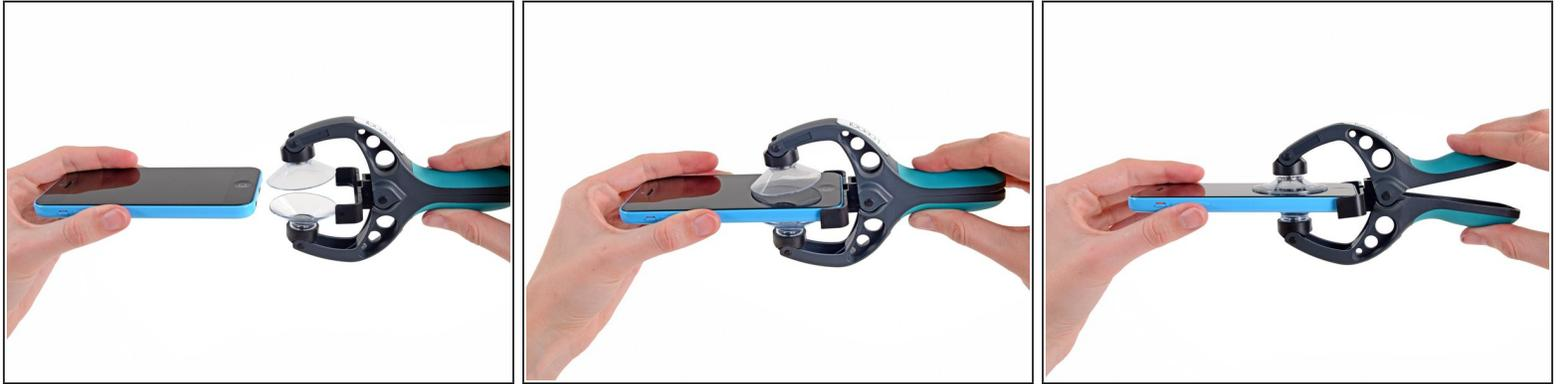
**i** The next two steps demonstrate using the [iSclack](#), a great tool for safely opening the iPhone 5c that we recommend for anyone doing more than one repair on an iPhone 5, 5s, or 5c. **If you aren't using the iSclack, skip to [Step 5](#).**
