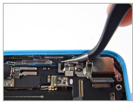
A small piece of tape may obscure the logic board grounding clip. If so, use a pair of tweezers to remove the tape.
