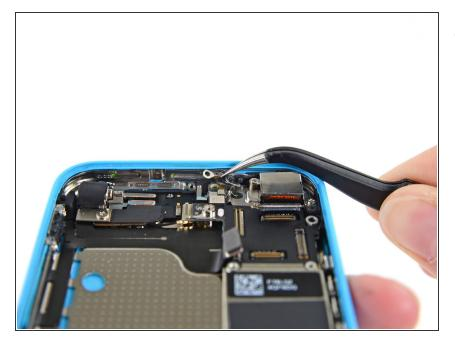
• Use tweezers to remove the logic board grounding clip.
