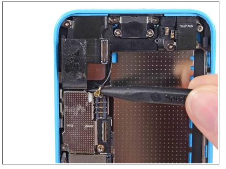
Disconnect the lower antenna connector from the base of the logic board.
