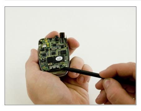
Carefully pry the logic board from the case with the spudger.
