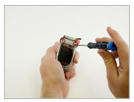
Remove screws with #0 Phillips screwdriver.
