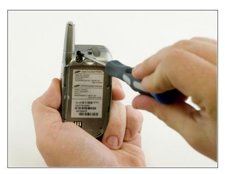
With a #0 Phillips screwdriver remove the screw which you just uncovered.
