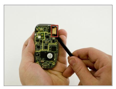
Gently pry up the ribbon-type connector with the spudger.
