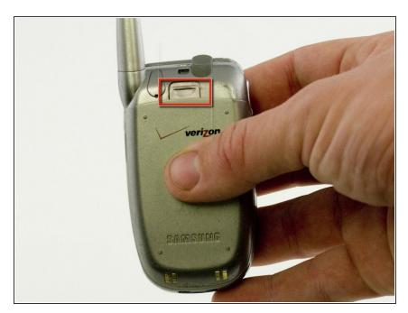
Slide the latch on the back of the phone up.
