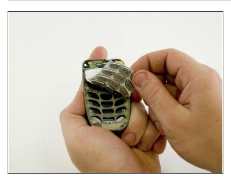
Once the logic board has been removed, peel the keypad up.
