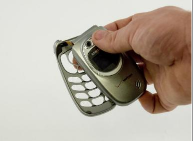
When using a spudger the keypad housing comes off quite easily, although it may be necessary to guide the ribbon cable through the slot in the housing.
