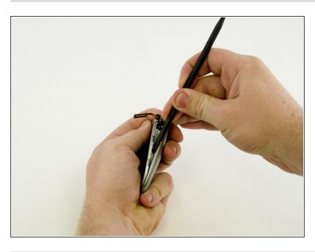
Carefully pry apart the casing with the spudger tool.
