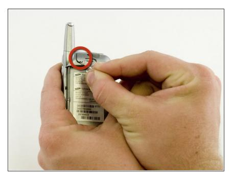
Using a thumbtack, pry the small plastic cover from the case near the base of the antenna.
