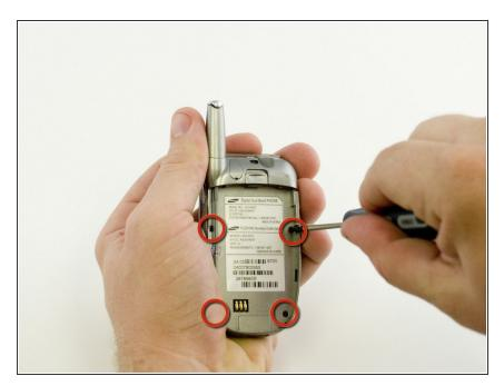
After removing the battery, remove the four small Phillips-head screws with a #0 Phillips screwdriver.
