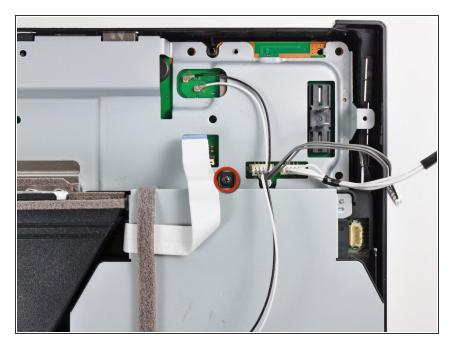
Remove the single 9.5 mm Phillips screw securing the Blu-ray drive to the lower case.
