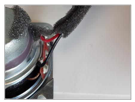
Remove about an inch of the black sponge insulation from around the red (positive) and black (negative) speaker wires.
