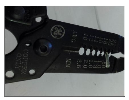
Strip about a quarter inch of the rubber insulation away from each of the speaker wires (red and black wires) using the 6 inch wire strippers.
