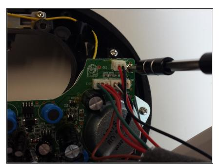
Remove the 4 phillips #1 head silver screws from the green circuit board.
