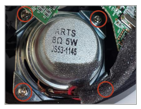
Remove the 4 silver phillips head #1 screws from the back of the speaker that are 7 mm in length.
