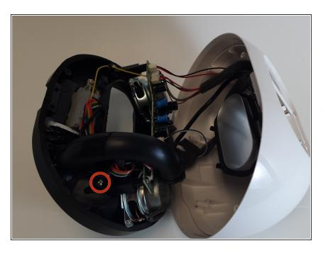
Remove the black tube (speaker port) by unscrewing the silver phillips head #1 screw (8 mm in length) that connects it to the black housing. Pull it off from where it wraps around the black housing's mating port.
