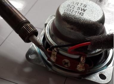
Use the soldering iron to heat up the terminal spots on the speaker and remove each wire (red and black).
