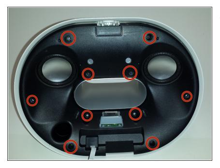
Remove the 10 screws from the black internal housing (6 black screws, 4 silver screws). They are all phillips #1 screws and the black screws are 10 mm in length and the silver screws are 8 mm in length.
