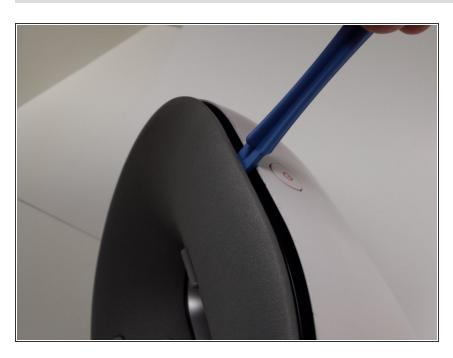
Pry off the front fascia by inserting a plastic opening tool between the fascia and white casing.
