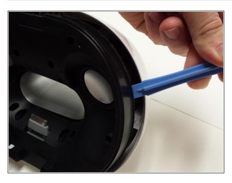
Slowly pry around the black housing with the plastic opening tool to remove it from the back housing.
