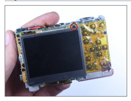
Remove the screw at the upper right corner of the metal housing.
