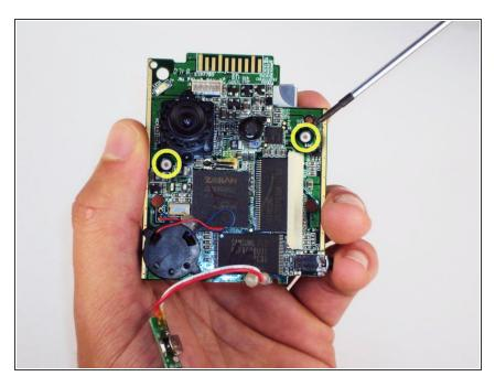
With the LCD screen facing away from you, remove the 2 bronze 3 mm screws securing the LCD using the #00 Phillips screwdriver.
