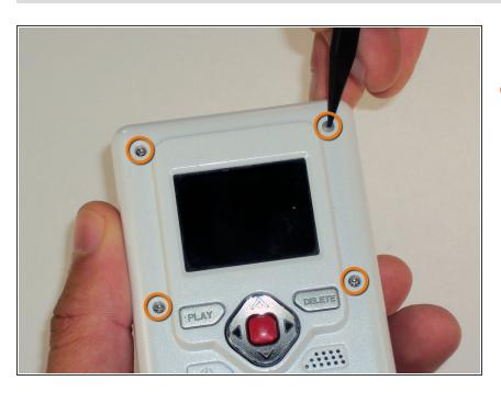
Remove the 4 gray screw caps with the spudger. These cover the screw heads and protect from dirt or grime.
