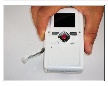
Open battery door. This can be done by gently depressing and sliding the battery down downward.
