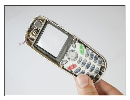
Put aside the back panel. You will only be working with the front panel from here on.
