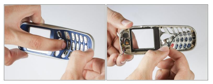
• Take out the key pad by pressing the keys on the face of the phone and pulling the rubber keypad from the other side.
