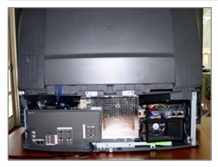
Remove the back panel from the television set. The panel runs the entire width of the bottom rear of the set. There's no need to remove the access panel for the lamp. That'll come off with the panel. There are 14 screws.
