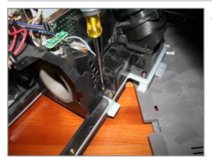
• Unscrew the color wheel cover. There are three screws holding it in place. One to the rear of the set, and two in front. The one to the rear is tucked way in, so I just unscrewed them and carefully left them in place and pulled them out with the cover. Slide the cover straight up, exposing the color wheel. As you do, note where the color wheel wires go — out the gap in the front.
