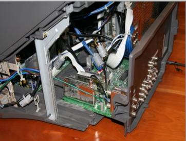
• Remove the panel on the left side by removing two screws holding it in place. Carefully slide it and the attached PC board out a few inches until cables stop you. You won't actually need to remove any cables from this board to get at the color wheel. (Of course I removed most of them the first time.)
