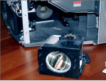
• Remove the projector lamp. This may be unnecessary, but (a) it let's you see your target (the color wheel) and (b) it just seems like the safe thing to do. It's easy. Just unscrew the two brass screws holding it in. It's on the right side of the TV. The screws won't come out, just pull them out with the whole unit by pulling on the handle and sliding it straight out. Carefully store it somewhere safe.
