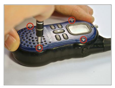
Remove the four 3 millimeter T6
