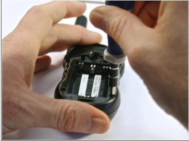
Remove the four 3 millimeter T8 Torx screws from the back of the radio.
