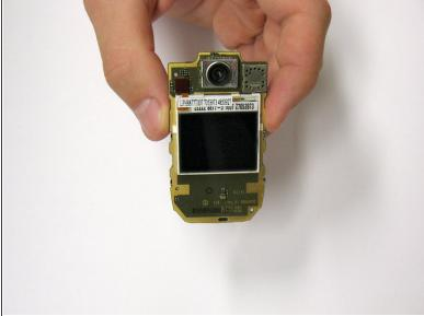
Pull out the circuit board, which will remove it completely from the case
