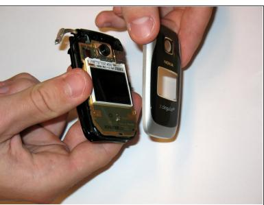
Keep the phone closed, and slide the lpod tool between the the silver and black phone case. Use the tool to slide all the way around the case to release the catches.
