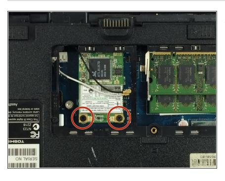
Unscrew the two 6 mm screws (indicated in red) located at the bottom of the WiFi card and store them in a safe place.
