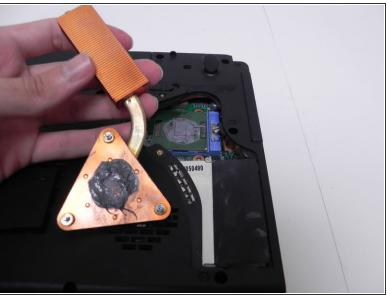
• Unscrew the copper heat-sink using a #1 screwdriver, and then lift it free. Do not get any thermal grease on any components. This part can now be replaced.
