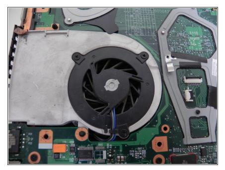
Follow the tear-down guide until you have access to the fan unit on the motherboard.
