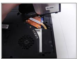
Remove the cover from the cooling unit.
