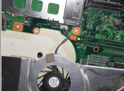
Unscrew the fan unit from the motherboard using a #0 screwdriver. Once the fan is unscrewed and unplugged from the motherboard, it can be replaced.
