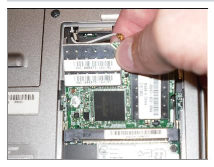
Lift the board up and out of the mini PCI slot at an angle of about 35 - 45 degrees
