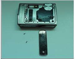
• Using the Phillips #00 screwdriver, unscrew the two screws on the side of the camera.
