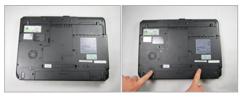
• Turn the laptop over and locate the lock and battery release switches. Unlock the battery by changing the switch on the right from locked to unlocked by sliding the switch outward.
