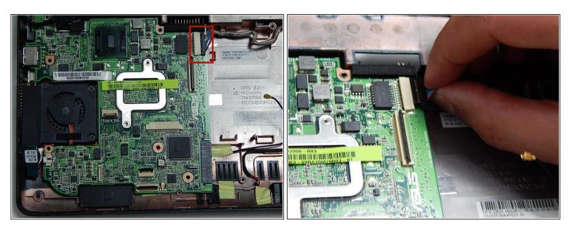
Detach the black structure connected to the input cables in the top right center of the motherboard by pulling them to the right, away from the fan.
