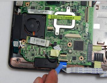
Detach the ribbon cable that connects the SD card module and the motherboard by lifting the black clips using the plastic opening tool.
