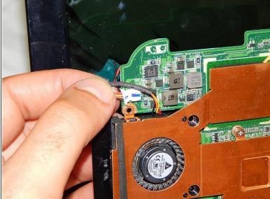
Disconnect the cable attaching the motherboard to the fan.
