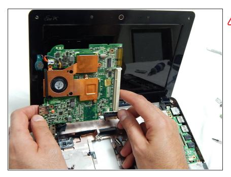
Gently lift the motherboard and hold it so that the bottom of the board is exposed.
