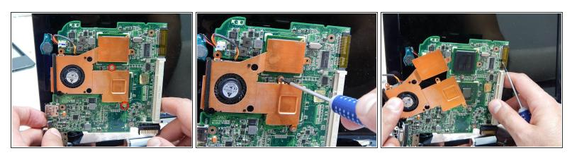
Remove two 5.5 mm screws holding the fan and the brass frame to the motherboard.
