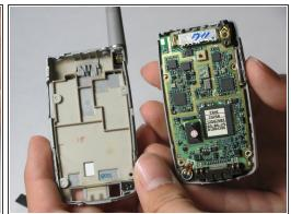
Carefully wedge the spudger around the sides of the plastic casing and pry off the back side of the phone.
