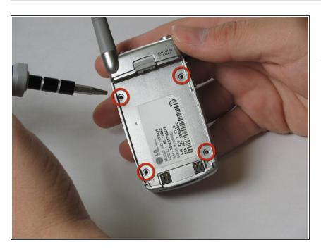
Use the T7 Torx screwdriver to remove the four screws that are in the cavity where the battery was.
