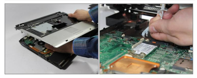
• Lift the top half of the case enough to get your hand beneath it, and then remove the two ribbon cables that connect it to the motherboard.
