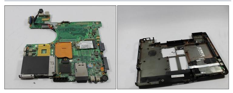
• Lift the motherboard out of the bottom case.
