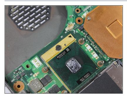
• Lift fan and heat sink out of case.
