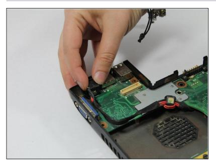
• Lift the power jack straight up and out of the slots that hold it in.
