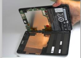
Pry open the left side of the case with a plastic opening tool. The backside of the tablet should now separate completely from the front.
