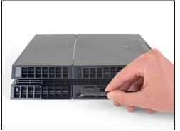
• Use <u>tweezers</u> to remove the two stickers in the center of the back of the PS4 exposing two case screws.
