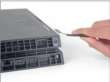
• Use tweezers to carefully remove the plastic screw covers in each corner, exposing two more case screws.
