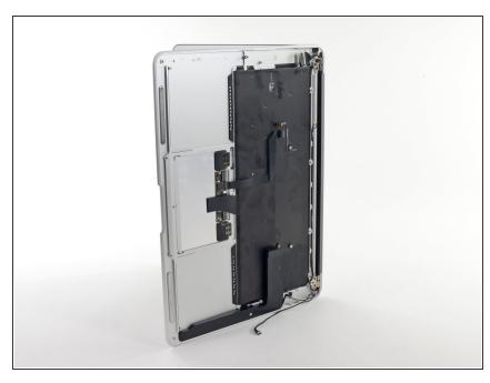
(i) Open the display so that it is perpendicular to the upper case and place it on a table as shown.
