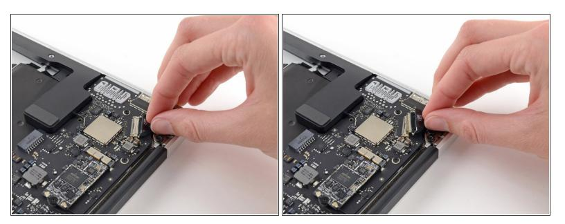
Pull the display data cable connector straight away from its socket.
