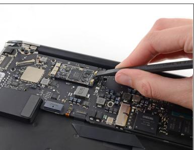
Use the flat end of a spudger to pry both antenna cable connectors up and off their sockets on the AirPort/Bluetooth card.
