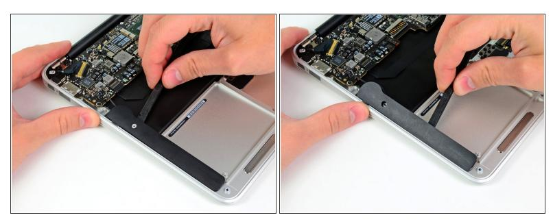
• Use the flat end of a spudger to pry the right speaker off the adhesive securing it to the upper case.
