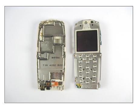
Pull the screen assembly from the base of the phone.
