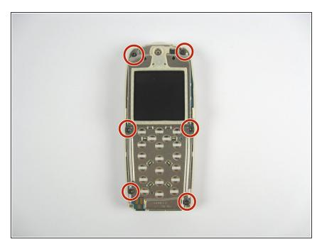
Remove the six screws along the edges of the phone.
