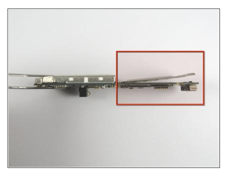
Carefully lift the keypad portion of the screen assembly from the circuit board.
