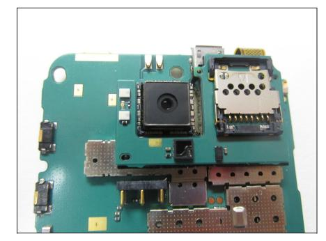
The camera can be popped out easily using a blunt knife or credit card. A new camera unit can be put into the same place. In case a Nokia N900 camera unit cannot be found, it is possible to use a Nokia N79 camera without causing damage.
