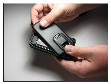
In the case that you do need a new back cover remove it by locating the slit on the side of the phone allowing you to take off the cover, but if you need to further get to your camera you will need to remove the back cover as well.
