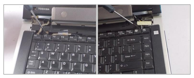
Remove both 6.72mm screws from the upper left and right of the keyboard using the Phillips #00 screwdriver.
