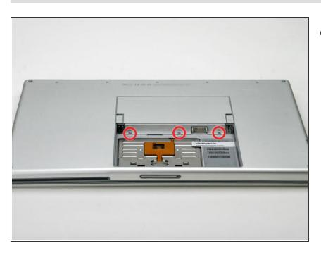
Remove the three identical Phillips screws from the memory door.
