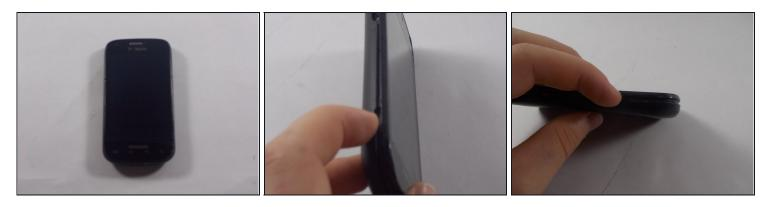
• Start by removing the back plastic cover by lifting it up from the notch on the left side of the phone
