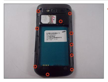
Remove the battery and use a small Phillips head screwdriver to remove the marked up screws
