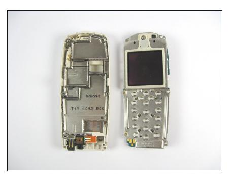
• Separate the screen assembly from the base.
