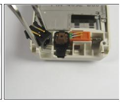
• Use a pair of tweezers to remove the DC input from the base.
