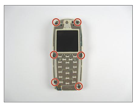
Using a T6 Torx screwdriver, remove the screws from the screen assembly.
