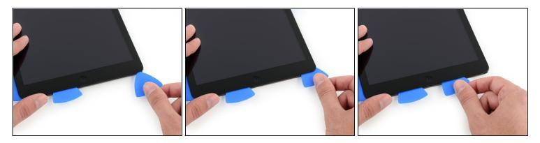
• With the adhesive loosened, you can now insert the pick near the right-hand corner. Slide the pick to the left, and stop just short of the Home button.
