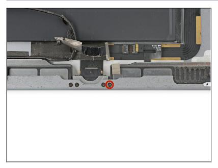
Remove the 2.2 mm Phillips #000 screw securing the speaker to the rear case.
