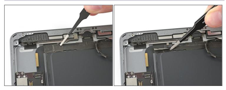
(i) A bend in the speaker cable makes it difficult to peel the tape up from the end.
