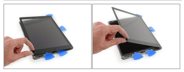
• Lift slowly and gently to further detach the adhesive along the display cable edge.
