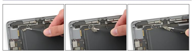
• Peel the tape toward the home button to uncover the speaker cable connector.
