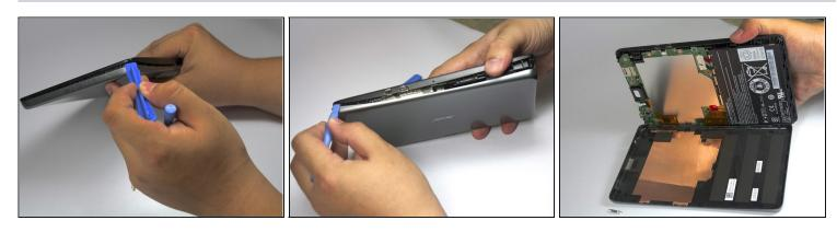
Pry open the left side of the case with a plastic opening tool. The backside of the tablet should now separate completely from the front.
