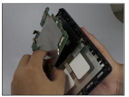
• After all ribbon cables are disconnected, move them out of the way, and the motherboard should fall out easily.
