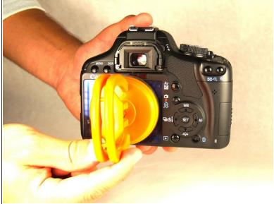
While holding the suction cup flat against the camera screen, suction the two together by pinching the orange handles to meet at the center.
