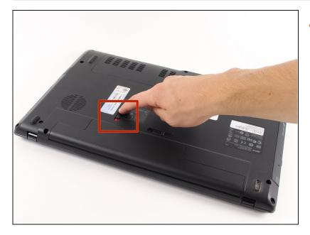
"Unlock" your battery by moving the switch as shown so that an unlocked lock on a red background is shown.
