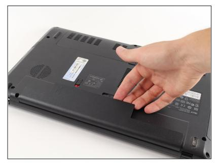
• Now remove the battery by lifting it out of the laptop by the side closest to the switches.
