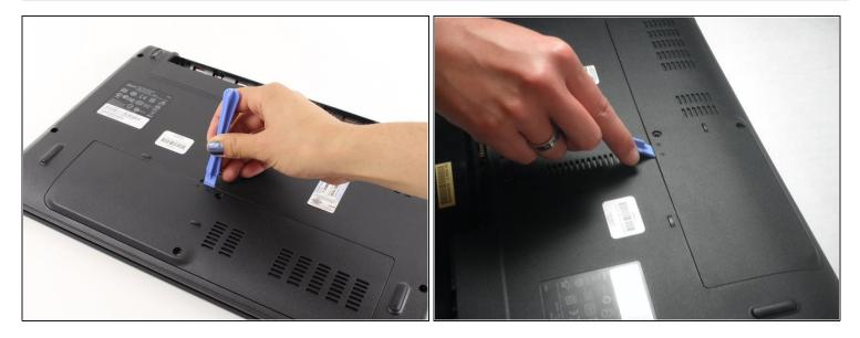
Once both screws have been removed use a plastic opening tool to lift the panel up. Starting
