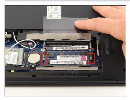
• Locate the two metal pieces on both sides of the RAM that are holding it in place.
