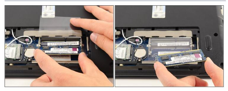
• Carefully slide the RAM out of the compartment.
