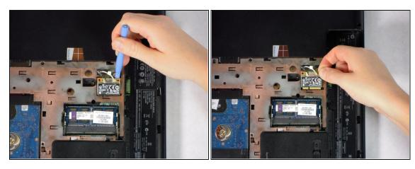
• Use a plastic opening tool to lift the wireless card out of its slot.
