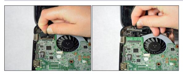
• In the top left hand corner, disconnect the monitor cable from the motherboard by pulling up on the black tab.
