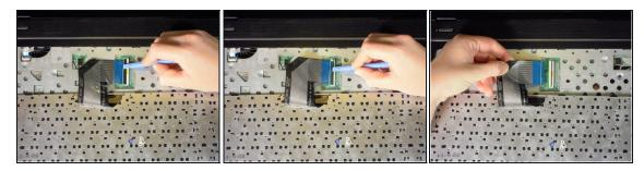
• Using a prying tool, flip the black clip up and to the right. Pull the silver cable out and to the left, the keyboard is now detached from the laptop.
