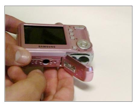
Slide open the battery compartment cover before removing the exterior covers of the camera.
